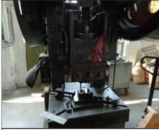
Photo of non-conformity NC-No machinery injury warning sign on punching machine.JPG
