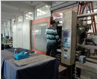
Photo of the inside of the main production hall Injection molding.JPG
